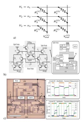
Fig. 15: a): Circuit of a MAC engine for analog SVM implementation. b): Schematic and layout of a 2-level analog Decision Tree with one root and two split nodes c): Digital post-processed image from multiple microscope photos of the printed 2-level analog Decision Tree with corresponding transient measurements.
