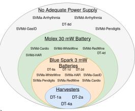
Fig. 19: Optimized analog and digital classifiers placed into sets based on which sources can power them (similar to Fig. 3). For each decision tree depth, we pick the set for the power source that can power all bespoke benchmark variants. E.g., Molex printed batteries can power depth-4 digital decision trees for each benchmark. Harvesters [42] are now capable of powering several decision trees. The 'a' and 'd' suffixes on 'SVM' and 'DT' are for 'analog' and 'digital' respectively.
