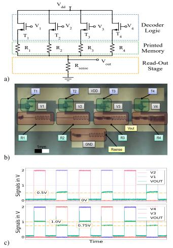
Fig. 14: **a**)/**b**): Schematic/Microscope Photo of a 4x1 ROM. **c**): Transient Measurements of the ROM.
