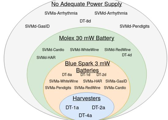
Fig. 19: Optimized analog and digital classifiers placed into sets based on which sources can power them (similar to Fig. 3). For each decision tree depth, we pick the set for the power source that can power all bespoke benchmark variants. E.g., Molex printed batteries can power depth-4 digital decision trees for each benchmark. Harvesters [42] are now capable of powering several decision trees. The 'a' and 'd' suffixes on 'SVM' and 'DT' are for 'analog' and 'digital' respectively.
