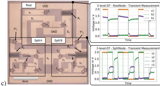
Fig. 15: **a)** Circuit of a MAC engine for analog SVM implementation. **b)** Schematic and layout of a 2-level analog Decision Tree with one root and two split nodes **c)** Digital post-processed image from multiple microscope photos of the printed 2-level analog Decision Tree with corresponding transient measurements.
